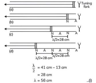
The next resonance should occur when the piston is pulled sufficiently far that a third node occurs, the other two nodes maintaining at their prior locations (Fig. d) Again, we have the given data:
